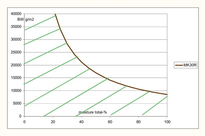
**Moisture accuracy for MK30R** - The moisture reading accuracy is dependent on the moisture level. The calibration performed will strongly affect and so do the measuring conditions.
