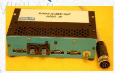
Cable with ITT Cannon and a Power Supply -PS having all connectors for communications and analog signals
