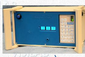
MK30R battery supported portable use with data saving and wireless transfer, fully self-contained, measuring head built-in. Measuring area diam. 40 mm, to depth 35 mm, range 4 - 95% of water
