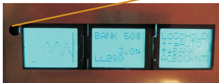
Figure 7. AK30 display with the trend curve and detailed information, in blueish colour in BANKS mode. The menu system is available at the same time.
