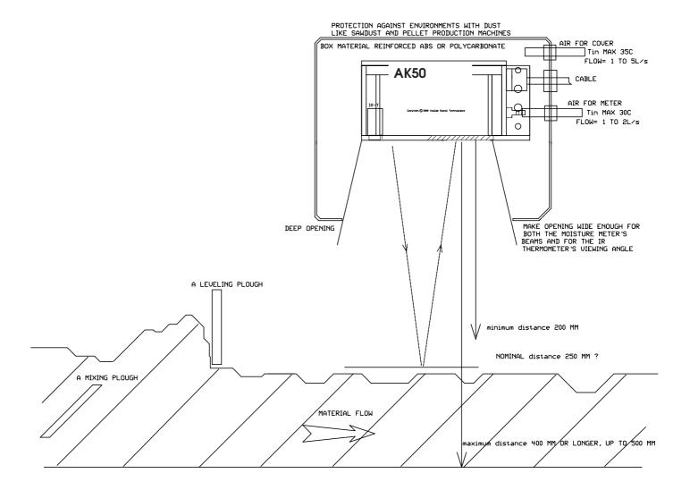
Figure 1. Protection against hot environments by using a standard box. An opening is machined or sawed to the bottom. Drawing is not to scale.
