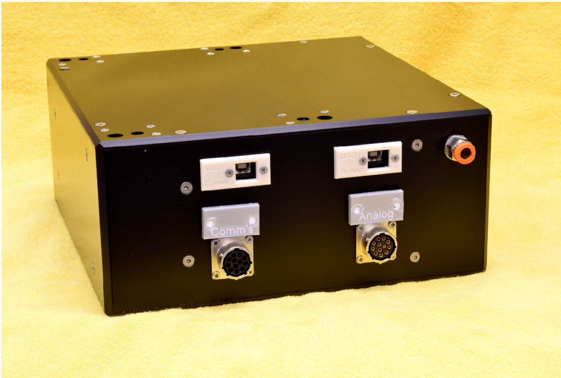
FrontColour 10 back panel for connections to power supply, communications, analog signals and USB. Top right corner has a quick connect for air purge
