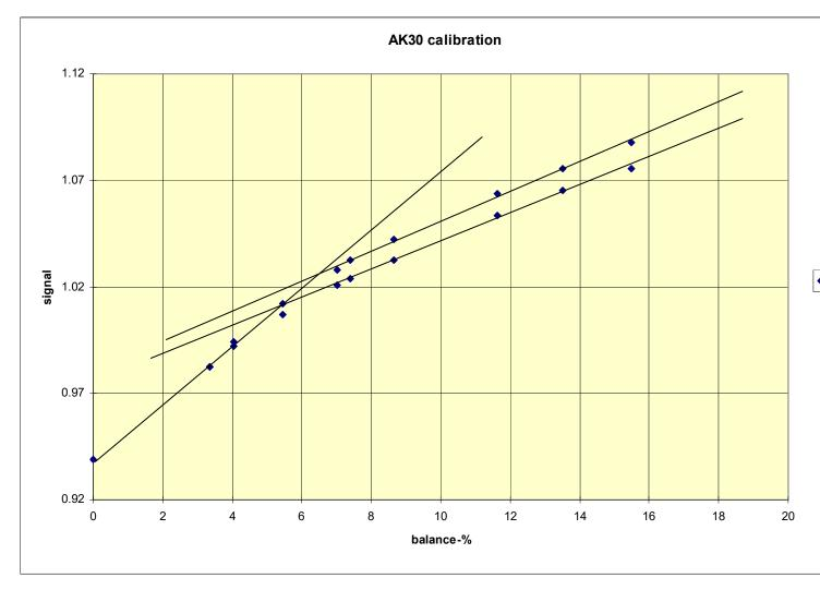
Figure 2. Calibration of a packaging paper
